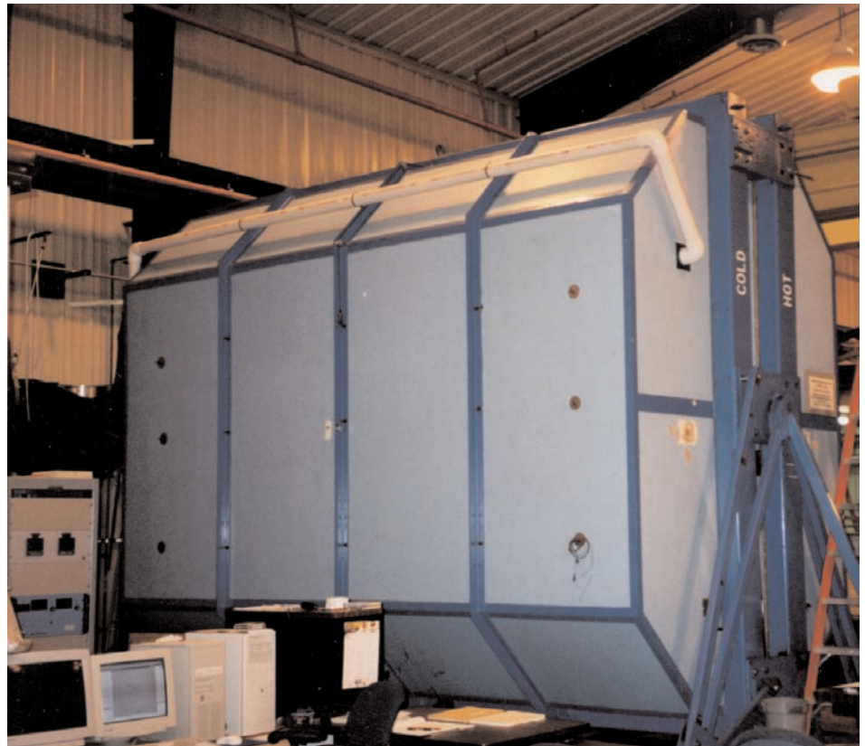
The ORNL whole wall testing chamber. (ORNL photo)
