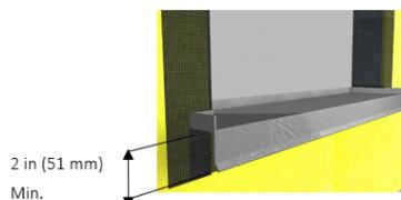
5. Sill Pan Flashing (Concealed) for use with nail-on-windows (refer to Dryvit Outsulation X Installation Details, DS837).
