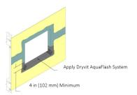
4) Install the specified component (i.e. window, etc.) and associated flashings per manufacturer's directions and contract documents. Then apply Backstop NTX – Texture or Smooth to the remainder of the wall surface as described in Section VI and lap over the previously installed material around openings – Figure 12..
