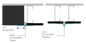
c. Using a brush or 3/4 in (19 mm) nap roller, apply a liberal coat of AquaFlash Liquid material to the backer rod and adjacent substrate surface to the width of the AquaFlash Mesh - Figure 15.
