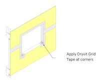
2) Using a stainless steel trowel apply Backstop NTX – Texture over the Grid Tape extending to the inside face of the opening and onto the face of the exterior sheathing a minimum of 6 in (152 mm) – Figure 10.
