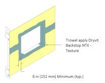
3) Apply Dryvit AquaFlash System at sill in accordance with Sections IV.A.3 and IV.C respectively. **NOTE: AquaFlash System must extend up the jambs a minimum of 4 in (102 mm) – Figure 11.**
