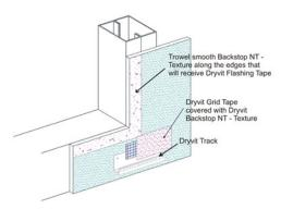
5) The Backstop NTX - Texture material should be applied in a uniform, continuous film at the recommended coverage rate. **NOTE: Substrates with a surface texture or high porosity will require additional material.**
