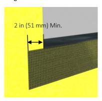
2) Begin at the sill of an opening. Using a brush or 3/4 in (19 mm) nap roller, apply a liberal coat of AquaFlash Liquid material to the air/water-resistive barrier/substrate surface.
