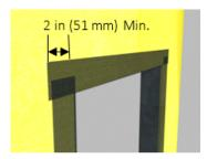
a) As an alternative, preformed Dryvit AquaFlash Corners can be applied at each corner of the opening to reduce the number of field cuts required. The AquaFlash Corners are installed in the same manner as the AquaFlash Mesh. – Figure 5
